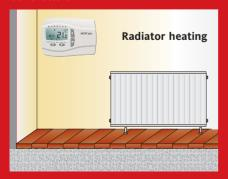
For controlling the room temperature (with optional remote sensor for measuring the room temperature)
