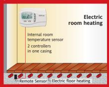
For controlling the room temperature and limiting the floor temperature to an adjustable maximum value (with remote sensor) for electric floor heating (direct heating)
