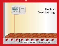
For controlling the floor temperature in electric floor heating systems, e. g. in bathrooms (with remote sensor)
